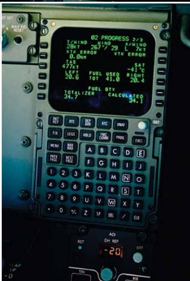
FMS Progress pages one and two, with a general overview of our flight and specific flight track and fuel information.
